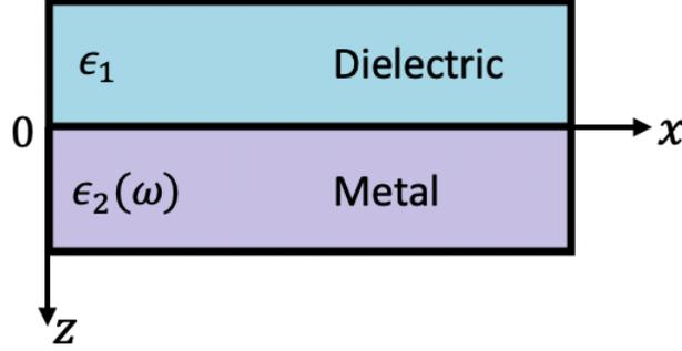
**Figure 3.1:** Illustration of the single dielectric-Metal Interface geometry with the corresponding axis convention, where the interface separating the two media is located at  $z = 0$ . The  $y$ -axis points into the paper and the system is assumed to be uniform along this axis.
